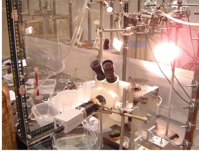
FIGURE 3. Photograph of the experimental setup for measuring contact angle in situ. This consists of a camera and microscope, with the substrate mounted on the SSLbL robot, illuminated from behind with a light.
