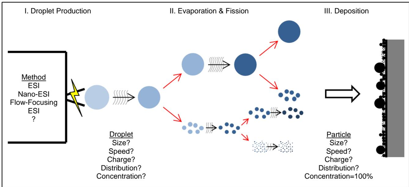
**Figure 1.** Schematic of a general ESI deposition method showing evaporation and droplet fission.
